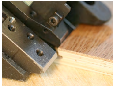
Fig. 18 Pushed in to the groove - correct position
