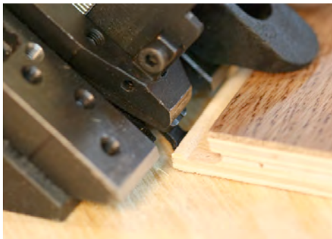
placed outside locking element - incorrect
