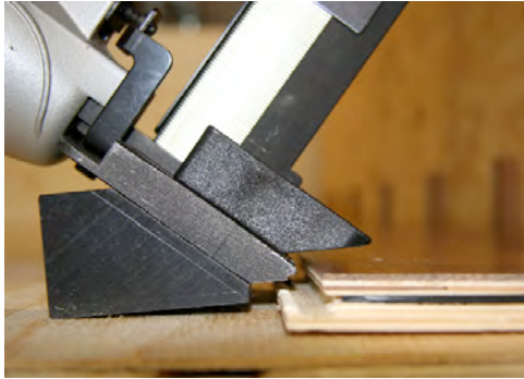
Fig. 13 – Lifting the staple gun over the locking element
